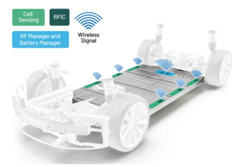
Analog Devices introduces the industry's first wireless battery management system for production electric vehicles (Photo: Business Wire)
